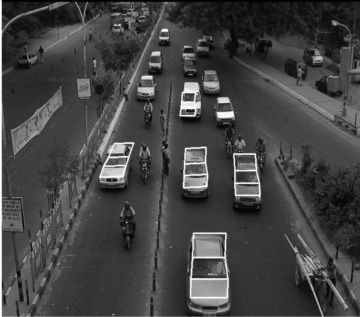
Result of 3D fitting. Notice the accuracy of localization of cars
