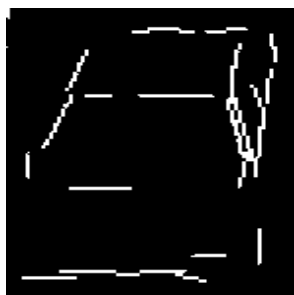
Edges extracted using Hough transform
