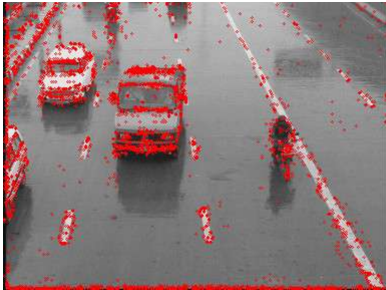
6191 keypoints left finally after rejection of keypoints which are not well localized.
